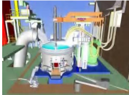
INTECO 60TEBT Electric Arc Furnace
