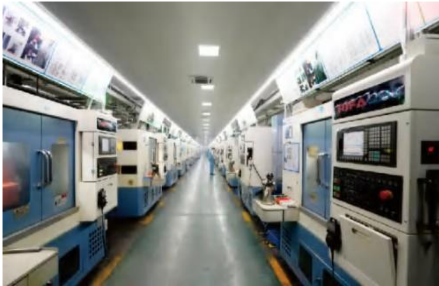
DGBB Auto grinding line
